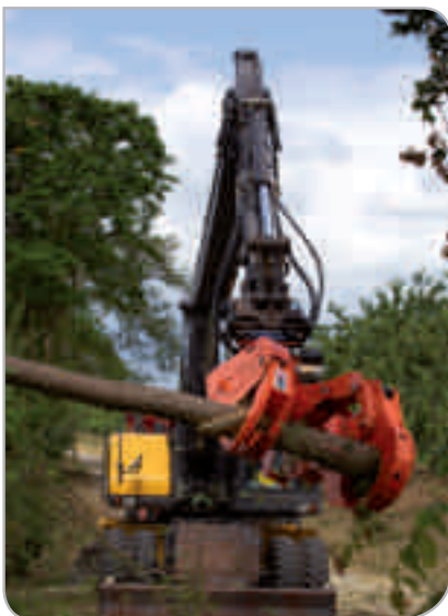
Mobile excavator with felling head.
